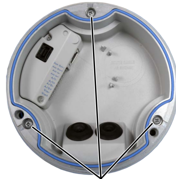
Twist-lock screws in back box
