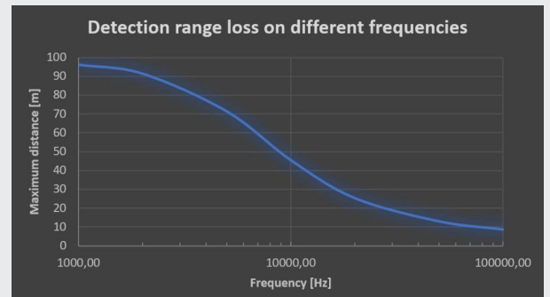
An example of detection range loss on different frequencies.
